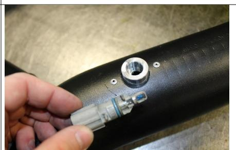
**9.3** Insert the breather crank case adapter 1403043-2 into the turbo inlet boot as shown and secure with a 32mm clamp (1302197).
