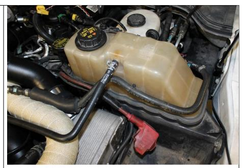
**9.14** Re-install the vacuum and coolant overflow lines into place on the driver's side and the heater line attachment.
