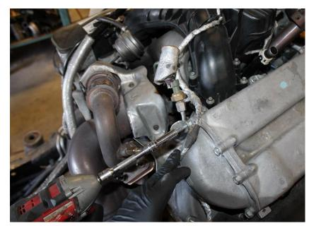
**R1.3** Using an 8mm socket remove the exhaust manifold to EGR upper exhaust tube from the cooler.
