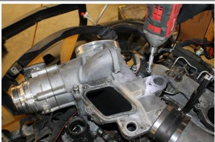
**R2.9** Using an 8mm socket, remove the 2 Coolant tube bolts and remove the tube. This completes the stock intake removal.
