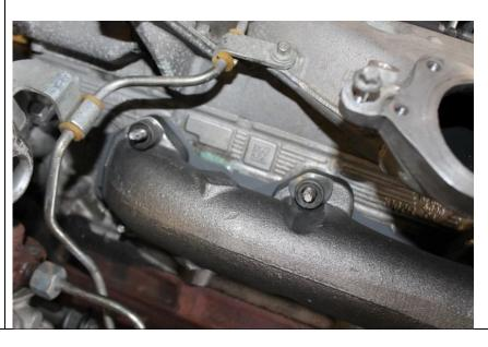
**2.3** Place the 1403002 BD heatshield into place on top of the front of the BD manifold.
