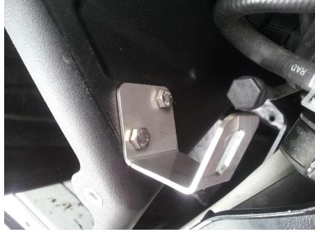
**10.5** Loosen and remove the Rad mount screw using a 10mm wrench.
