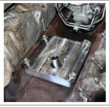
**1.3** Torque down the 4 pedestal block off plate bolts using a 13mm socket to 41 ft. lbs.
