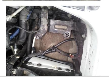
**10.7** Remove the OEM rubber air box mounts and install the 2 1456737 M8 U nuts as shown onto the air box mount.
