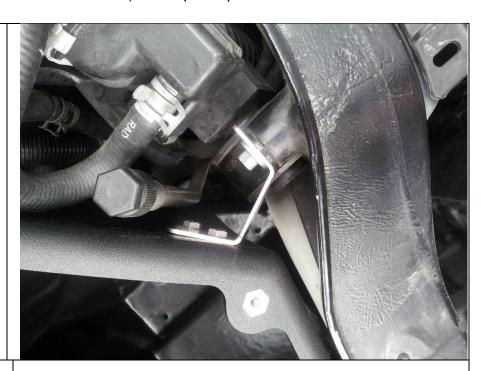
**10.10** Install the 1453820 seal onto the air box outlet hole if it has not been installed already.
