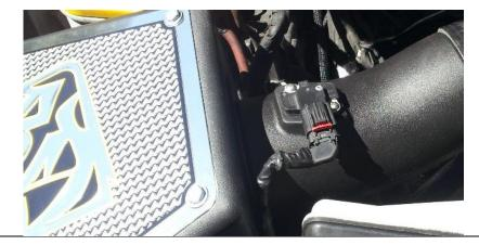
**10.14** Install the air box lid with the 1405422 M6 Stainless Screws. This Completes the intake section install.
