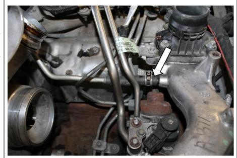
**R4.3** Pull the turbocharger off at this time. Lift up and towards the rear of the engine.
