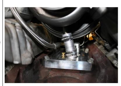
**3.15** Use a small amount of pipe sealant or teflon tape on the threads and install the Oil Feed 90° fitting 1462321 into the CHRA Oil inlet. Do not use excessive amounts of sealant, as this could cause oil contamination.
