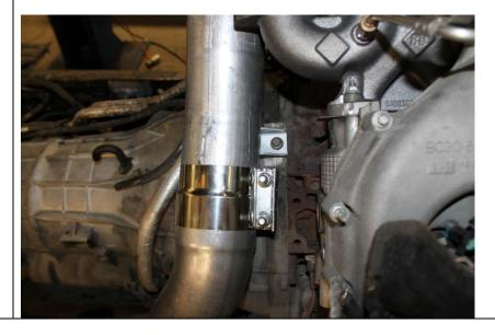
**6.2** Slide the laser cut Lower downpipe flange 1403017-2 onto the lower downpipe 1403017-1.
