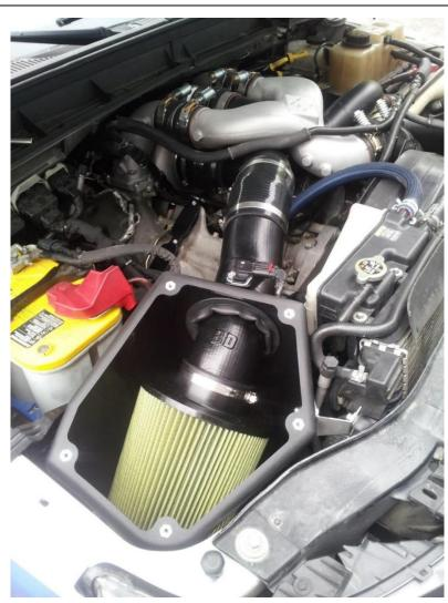
**10.13** Tighten the air filter clamp to the intake tube at this time.
