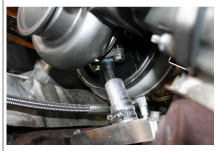
**3.14** Tighten the oil drain hose gear clamps at this time.
