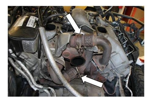
R3.5 Using a 13mm socket, remove the 6 nuts fastening the up pipes to the stock exhaust manifolds, penetrating oil can be used to aid in the removal of these. This completes removal of the exhaust system except for the passenger side manifold which will be done after the turbo has been removed.
