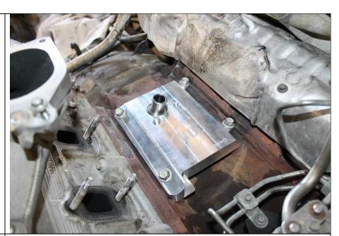
**1.4** Install a 1/8" NPT plug in the water feed location unless you are installing an aftermarket watercooled wastegate or non-standard watercooler CHRA turbocharger. Use a thread sealant such as Permatex or teflon tape. Insure the NPT is well seated.
