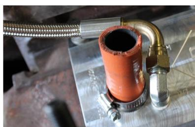
**3.7** Tighten the 1453113 gear clamp to secure oil drain hose.
