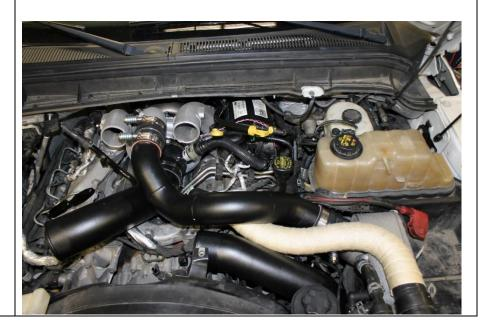
**9.13** Place 2 3" Boots 1405305 onto the intake horns and slide the 1401563 3.5" boot onto the Y pipe end. Install the Y pipe into position as shown. All clamps can be tightened down until spring bound.
