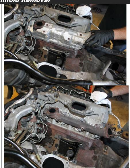
**R.2** Using a 13mm socket, remove the 8 main manifold nuts. Some studs may come with these and will need to be reinstalled after manifold removal. The manifold can now be removed from the passenger side head. If any studs were removed reinstall these and torque to 115 lb-in.
