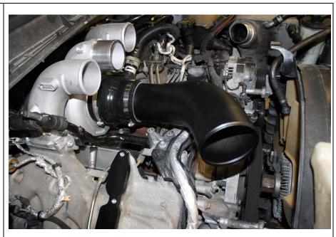
**9.7** Install the only 1407030 clamp provided in the kit for the intercooler and 3.5" clamps as shown on to the 3.5" CAC Tube. Adjust so they are held from rotating but are movable.
