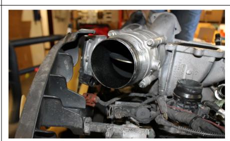
**R2.7** Using an 8mm socket, loosen the front and rear intake boots to the turbo, these boots can be detached when the turbo has been removed.
