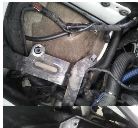
**10.8** Place the air box in position and install the 1456738 M8 bolts.
