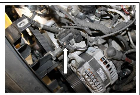
**7.6** Remove the wastegate actuator solenoid and the vacuum tubing lines routed both toward the driver side and passenger Side at this time. Remove the 2 bolts with an 8mm socket. The harness and plugs related to these items can be zip tied and taped up / sealed if wished.
