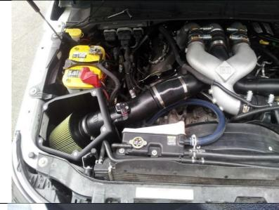
**10.14** Install the OEM MAF sensor into the intake tube as shown, use the provided 2 x 8-32 FT-0173590 and 1403041-1 gasket.
