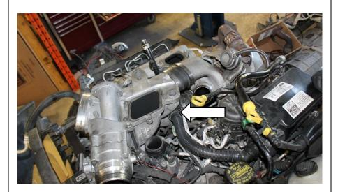
**R2.6** Unplug the intake throttle body plug located at the front of the lower intake.
