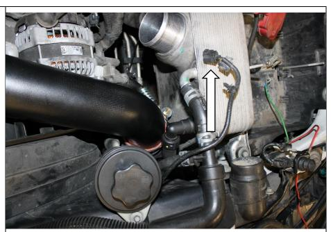
**9.11** Install the OEM upper coolant line, if your heat wrap has been damaged we recommend a new coolant tube or wrapping with a header wrap or similar high temperature insulator. Assure the OE clips snap into place.
