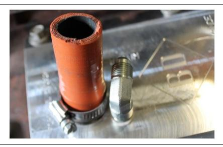
**3.6** Install the oil feed tube 1453130-B into position with the 90° section installed on the lower section as seen in the photo.
