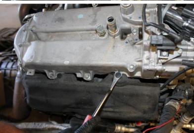
R1.6 Using an 8mm socket remove the 7 bolts holding the EGR cooler to the passenger side head. The EGR cooler can now be removed from the engine. Note coolant will still be present in the cooler as you remove it.
