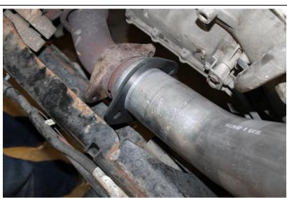
**6.3** With the flange sitting on the tube, install the lower downpipe into position along with the intermediate 4" lap exhaust clamp 1100740.
