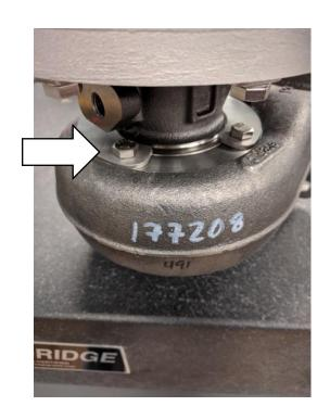
**3.2** The compressor cover bolts can be slightly loosened to allow it to be clocked into position once installed. Only loosen until the compressor cover can be rotated with some force and is still held in position.
