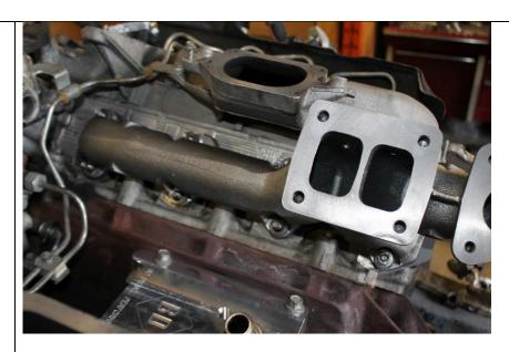
**2.2** Place the T4 flange 1403000 BD manifold into place on the passenger side head. Install the OEM Ford spacers onto the studs after the manifold has been positioned.
