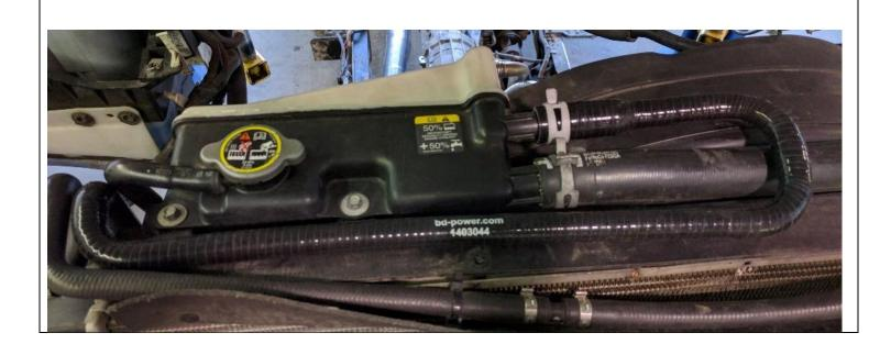
10.2 Route the coolant line around the radiator and other factory lines and connect to the radiator. Secure with the spring clamp (1302198).
