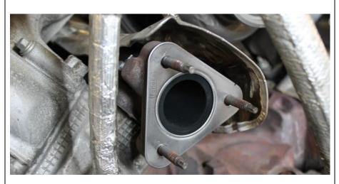
**5.2** During this section assure the transmission dipstick is on the inside or front of the cross over tube. It will need to be massaged into shape to clear in the following step.
