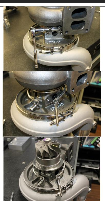
**3.2** The compressor cover V band clamp can be slightly loosened to allow it to be clocked into position once installed. Only loosen until the compressor cover can be rotated with some force and is still held in position.
