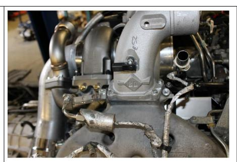
**7.3** Plug the harness into the MAP sensor and zip tie the harness as necessary away from heat sources and from wear due to vibration. The VGT actuator plug can be tapped up or capped.
