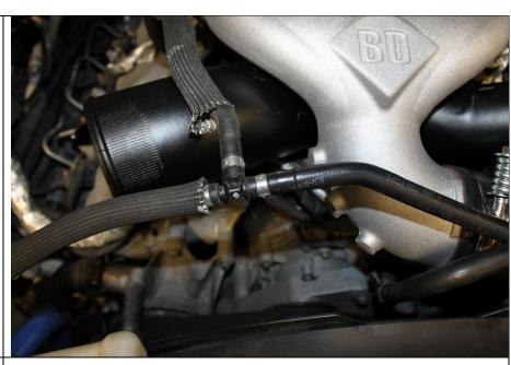
**9.16** Install 1900067 5/16" barb using the supplied CTL-8.5 as shown.
