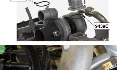
4.2 Install the driver's side intake into place first using the 4x M6 bolts 1900056 and a 10mm socket.
