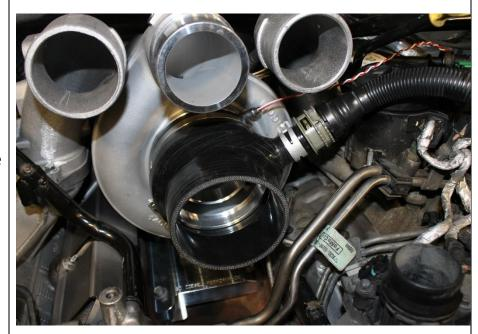
**9.6** Place the 4" Intake Tube Into position as shown, with 1453701 gear clamp installed on the 4-5" intake boot. Do not tighten the gear clamps at this time.
