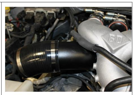
10.12 Place the 1401604 air filter into the air box before installing the 1403041 rotary molded intake tube. Slide the tube on an offset just behind the 22° boot. Seat the tube into the air filter as you slide it into place. The 22° boot outlet end can then be seated. Align the tube and boot into position and tighten all clamps.
