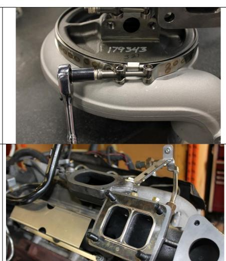
**3.3** Place the 2475042 T4 gasket onto the manifold.
