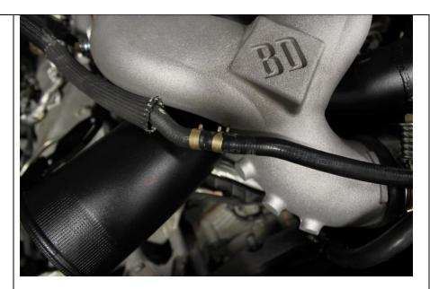
**9.17** Join the sections and clamp with a CTL-8.5 clamp. Slide the stock hose covering overtop of the clamps and place the hose as shown. Reinstall the clamp at the heater coolant fitting near the passenger side intake horn.
