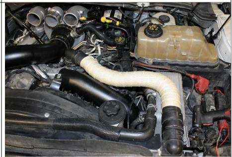
**9.12** Install the 3" Hot side CAC Tube 1403031 with the specified boots and clamps. Place the T Bolts on the bottom side and pointing towards the passenger side. All clamps can be tightened down until spring bound.
