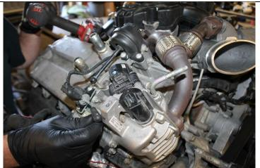
**R1.2** Using a 10mm socket & 16mm wrench remove the EBP sensor and tube at located at the rear of the EGR Cooler. Place the sensor and tube aside this will be reused in the BD Install procedures.
