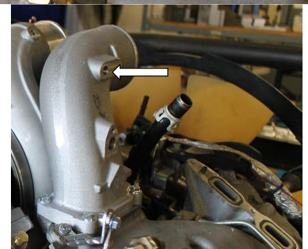
4.5 The compressor cover can now be clocked in position with the outlet centered between the two intake horns. Tighten the bolts to 120 in-lbs.
