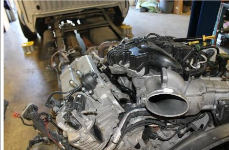
R1.5 On the passenger side of the engine, remove the upper clips from sound dampening shield. These are mounted to the EGR cooler and will need to be released to remove the cooler.
