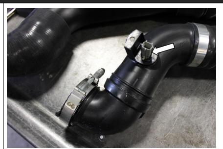
**9.2** Install the OE IAT into the BD CAC Tube 1403032-1. Rotate until the clip locks into place as shown.
