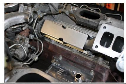
**2.4** Install the OEM manifold nuts and torque to first pass at 15ftlbs.
