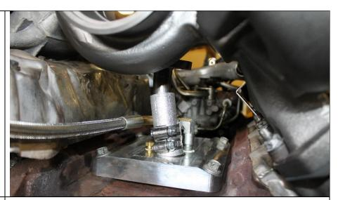
**3.10** The 148062 oil drain gasket can be placed in position now for when the CHRA is installed, or it can be slid into position after the CHRA is installed.
