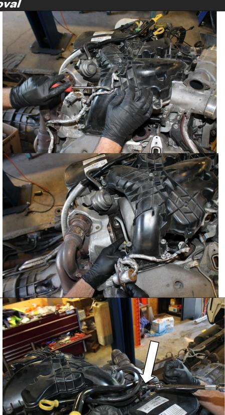
**R2.2** Using an 8mm socket remove the two bolts holding the two dipsticks to the intake on the driver's side.
