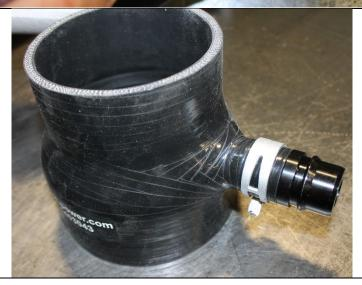
**9.4** Install the assembled intake boot onto the Turbocharger at the shown angle. Place the gear clamp in the shown orientation.
