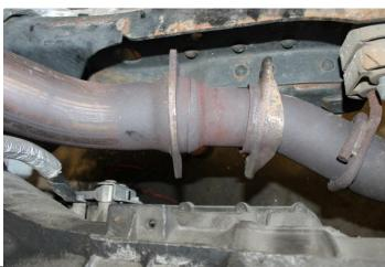
**R3.2** Using a 10mm Socket, remove the bolt holding the OEM cobra downpipe, this is found at between the rear of the engine and the upper down pipe.
