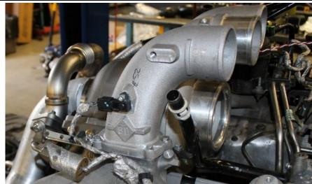
7.4 We recommend removing the plastic wire harness support bracket shown, this will clean up the install as it has no mounting locations with the EGR Cooler not in place. Arrange the wire harness as required and assure it's not free to vibrate and wear on sharp edges.
