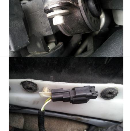
**10.6** If equipped remove the second alternator hook up plug seen on the front of the battery tray and secure out of the way of the new air box attached to the harness below.
