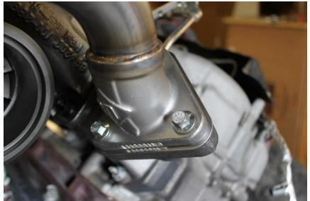
**5.3** Torque the cross over tube bolts and nuts to 18 ft. lbs.
